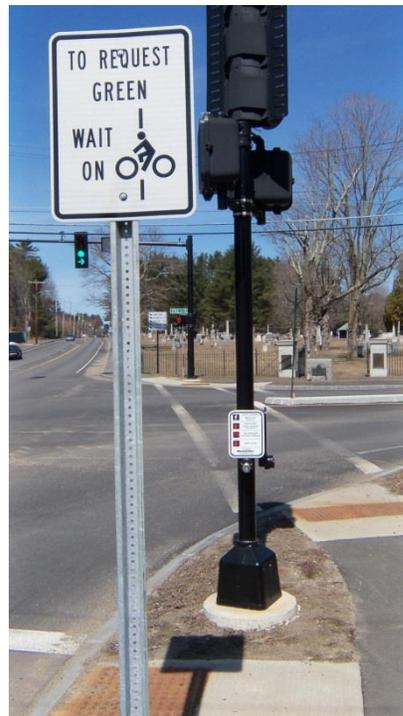
The new traffic signal at the N. State/Sewalls Falls intersection can detect and respond to bicycles when they stop at a designated spot in the bike lane.
